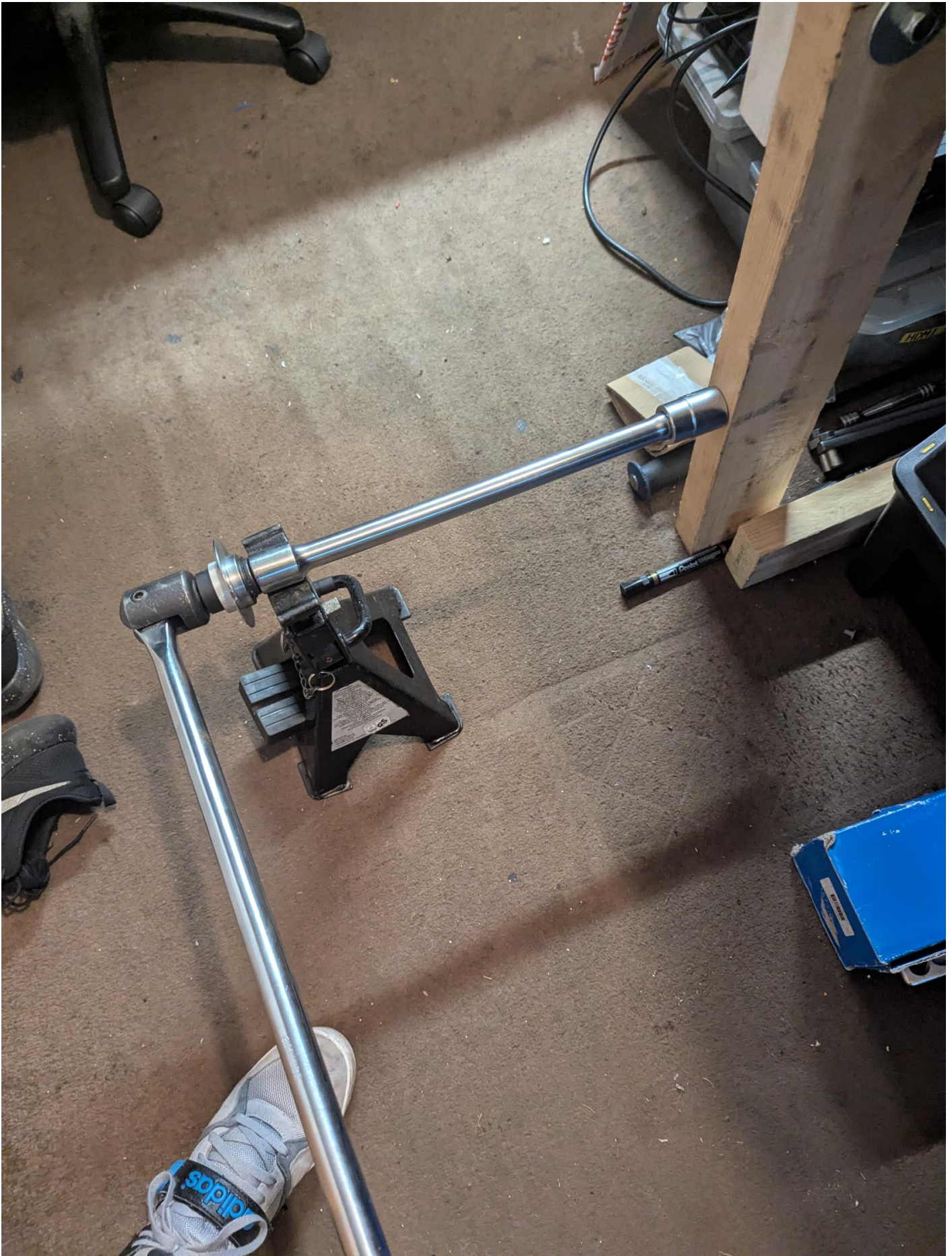
10. Using a 6mm Hex loosen the 4 small bolts around the crank bolt.
